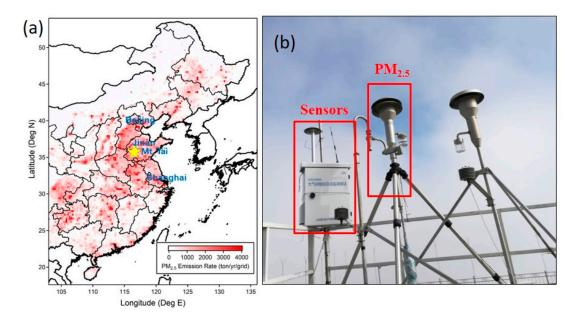
**Figure 1.** (a) Map showing the location of Mt. Tai. The emission data of fine particulate matter (PM<sub>2.5</sub>) were downloaded from http://meicmodel.org/about.html. (b) Photo of the sampling inlets of the air quality sensor and benchmark instruments on the rooftop of Mt. Tai station.
