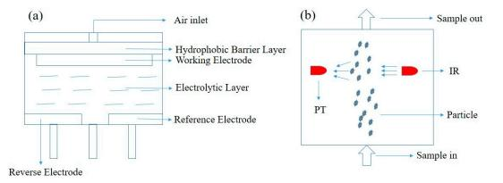
**Figure 2.** Schematic diagrams of the sensors evaluated in this work: (**a**) CO and O<sub>3</sub>, and (**b**) PM<sub>2.5</sub>. PT: Photodetector.
