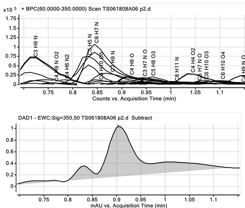
**Figure 7.** MS, Extracted ion chromatogram (EIC) and UV/Vis detector chromatogram (DAD1) for the same 19 June 2008 cloud water sample zoomed to the first minute. The mass spectrum was acquired using positive mode electrospray ionization. There is no obvious correlation between MS and absorbance detector signals. The MS chromatogram was time corrected to account for the time needed for the sample to pass between the UV/Vis and MS detectors.
