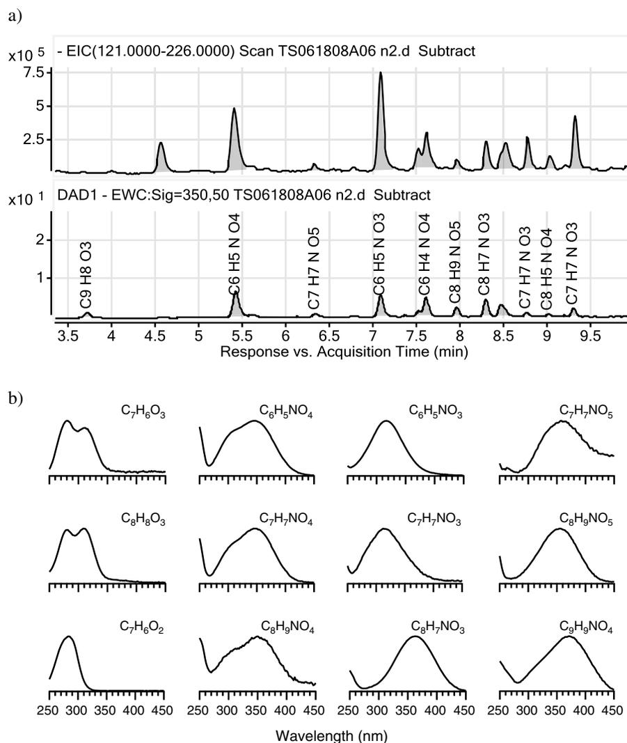
**Figure 3.** (a) MS, Extracted ion chromatogram (EIC) and UV/Vis diode array detector chromatogram (DAD1) for the cloud water sample collected during the biomass burning-impacted event on 19 June 2008 (TS061808A06). The mass spectrum was acquired using negative mode electrospray ionization. (b) Extracted UV/Vis spectra for selected peaks with assigned elemental formulae.
