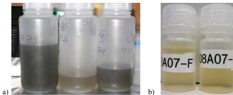
**Figure 1.** (a) Photograph of unfiltered cloud water samples collected at Mt. Tai on 19 June 2008. From left to right, the three bottles contain bulk, large drop, and small drop samples, respectively, (b) Photograph of filtered cloud water samples from the same date.
