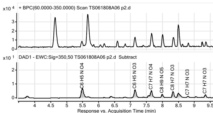
**Figure 6.** MS, extracted ion chromatogram (EIC), and UV/Vis detector chromatogram (DAD1) for a cloud water sample collected during BB event on 19 June 2008. The mass spectrum was acquired using positive mode electrospray ionization.
